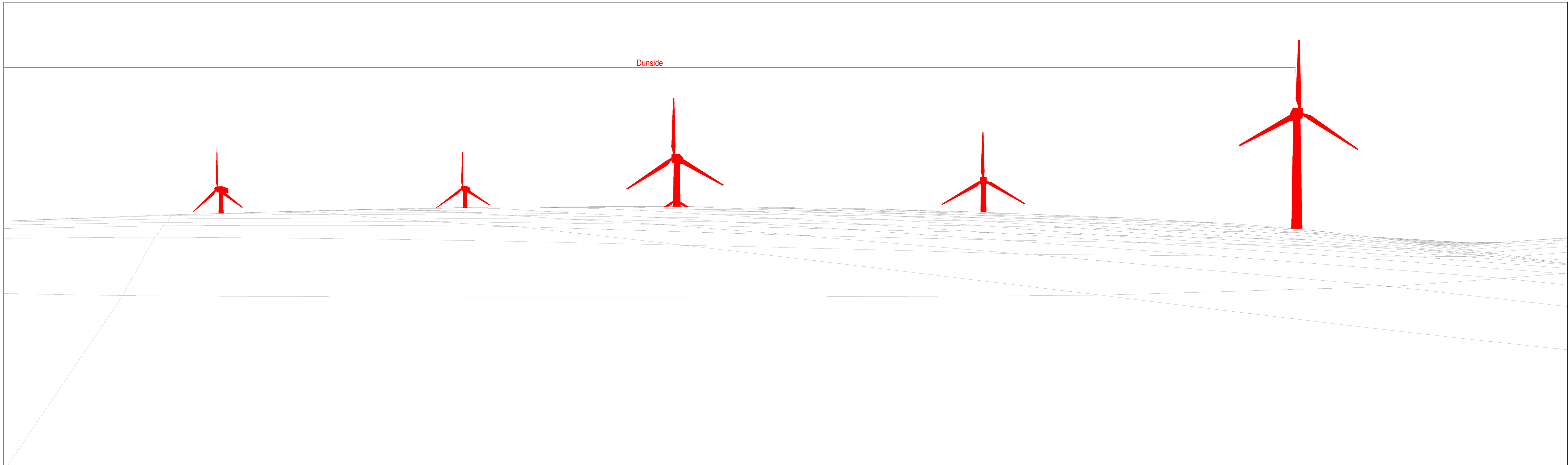
Wireline drawing - Showing proposed Dunside turbines with Hub height of 139m, Rotor Diameter of 162m, Tip height of 220m The view horizon has been lowered in this image to allow a greater visible vertical extent of turbines to be shown
